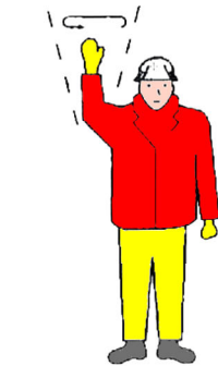
HOIST Clench and unclench fingers to "inch" load
